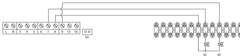
Collegamento valvole per impianti a 4 tubi (4T) Valves connection for 4 pipe plant (4T)
