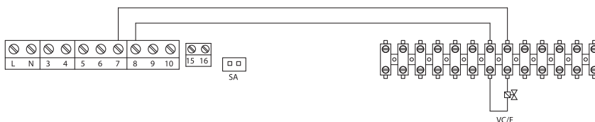
Collegamento valvole per impianti a 4 tubi (4T) Valves connection for 4 pipe plant (4T)
