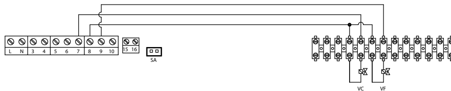
Collegamento valvole per impianto a 4 tubi (4T) Valve connection for 4 pipes plant (4T)
