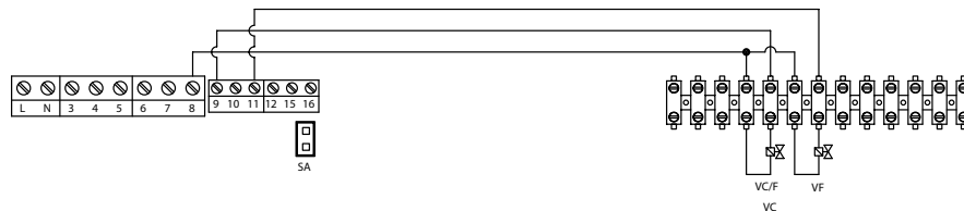
Collegamento valvole per impianto a 2/4 tubi (VC/F x 2T - VC + VF x 4T) Valves connection for 2/4 pipes plant (VC/F x 2T - VC + VF x 4T)
